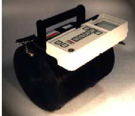
Fig. C.1. Victoreen neutron survey meter Model 190N.
